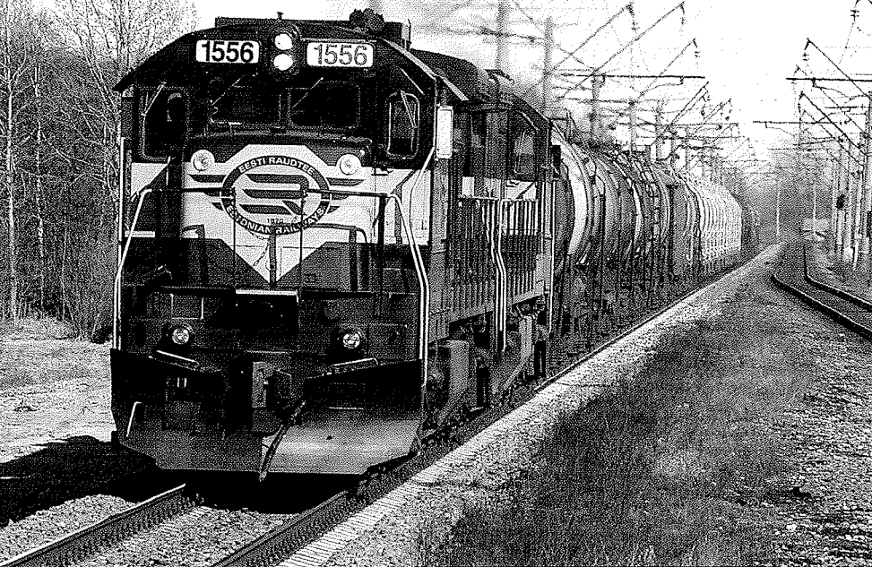
ABOVE: A pair of C36-7i Ges, Nos. 1556 and 1526 (former UP 633 and 7967 built in 1985) pull hard uphill on the approach to Kehra on the evening of 21 April 2003 with a westbound train consisting mainly of oil tanks.
