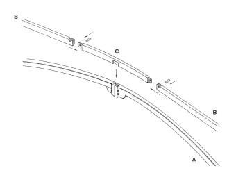
Figure 7: A line drawing showing the relationship between the component parts. Part A is the upper rib, B is the two main bearers per frame and C is the crown bearer. (Shelley White)
