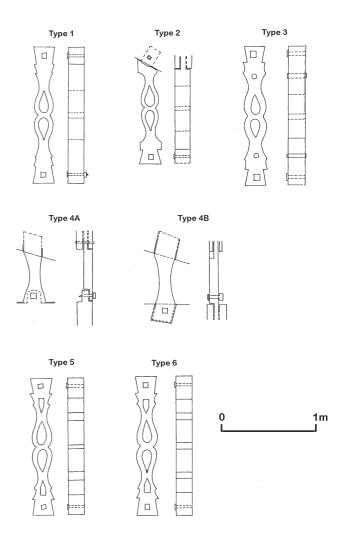
Figure 9: The typology of upper and lower radials
