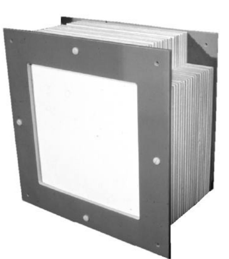
Figure 9. Realisation of a negative epsilon structure: photograph of the structure shown in figure 8. The aperture is 200mm×200mm.
