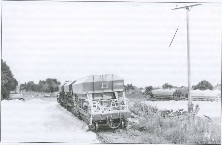
A quiet day at Greenisland - loaded wagons on the Down line and No.3 awaiting instructions on the Back line with not a soul in sight except the fireman. The tail pipe and vacuum brake application valve can be seen on the rear of the nearest wagon. [C Friel]
