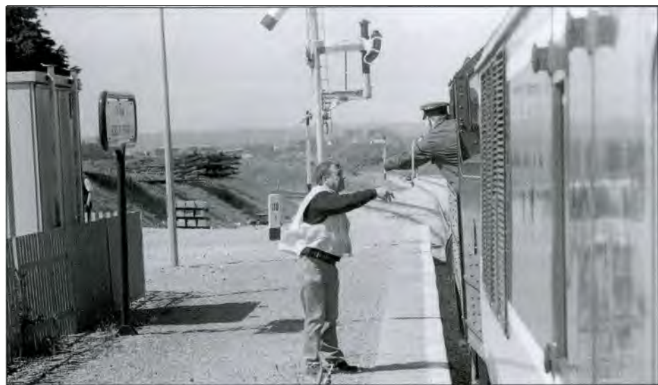
On the Rosslare Harbour-Waterford leg of the "Suir Valley" No.4 is about to leave the Dublin line at Rosslare Strand. The signalman handing up the new token is keeping things at arm's length, but the one arriving from the Harbour seems about to get him in the leg! [C Friel]
