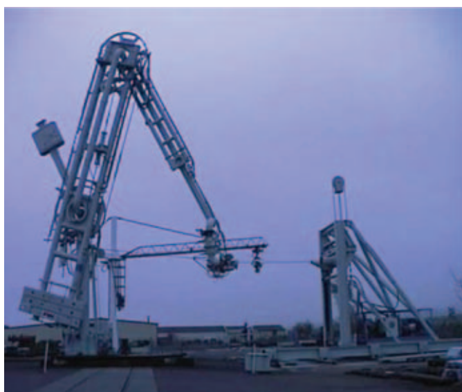
Figure 4.8 Full scale LNG loading arm testing rig
