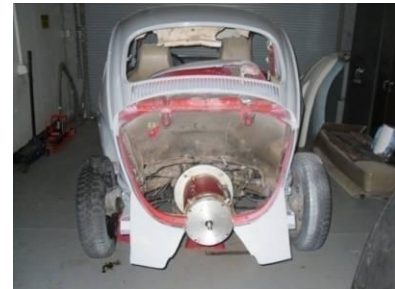
Figure 10. Electric motor coupled to original transmission.
