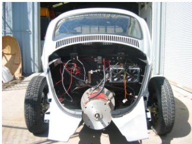
Figure 16. Motor controller, battery charger installed and system wired.
