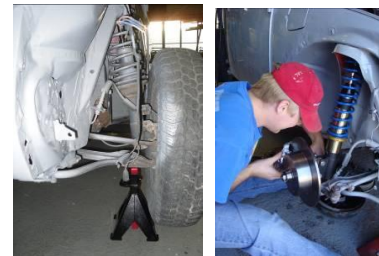
Figure 11. Suspension upgraded and disc brakes installed.
