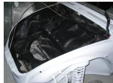
Figure 12. Interior cleaned and painted in preparation for final installation of components.
