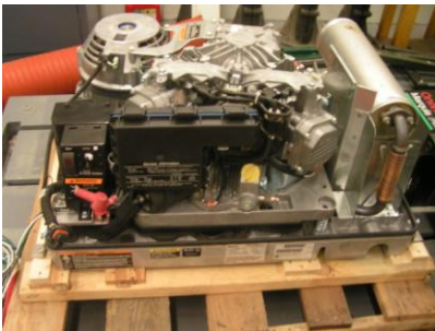
Figure 15. Gasoline generator being retrofitted to run on ethanol for eventual incorporation in vehicle.
