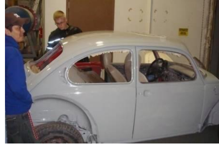
Figure 8. Vehicle was primed and moved into workspace.
