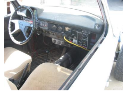
Figure 17. Generator control moved inside the vehicle and gauges added.
