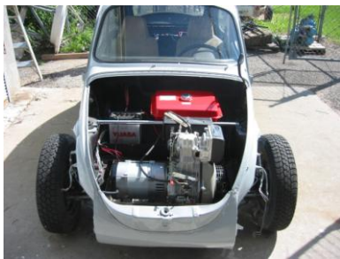
Figure 14. Generator implemented to run 100% biodiesel recycled from used cooking oil in campus dining halls.
