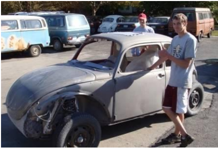
Figure 6. Vehicle was sandblasted to remove old paint.
