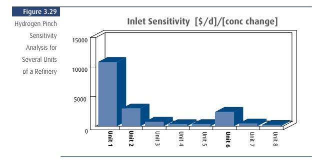
The application of *inlet sensitivity analysis* to hydrogen systems is normally performed to identify the units where an increase in feed purity is the most profitable (purer hydrogen can produce benefits on production, but there is a cost to obtain this higher purity considering the purity and pressure levels available on the site). This approach potentially has the largest overall benefit in terms of hydrogen cost and production improvements.
