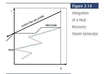
In the opposite situation, when the process requires more heat/steam than is available from the flue gas coming out of the gas turbine, an afterburner may be required to increase temperature levels at the exhaust of the gas turbine. The spent air issuing from the turbine still contains oxygen and may be fed through a second burner in order to supplement the heat available in the exhaust gases.
