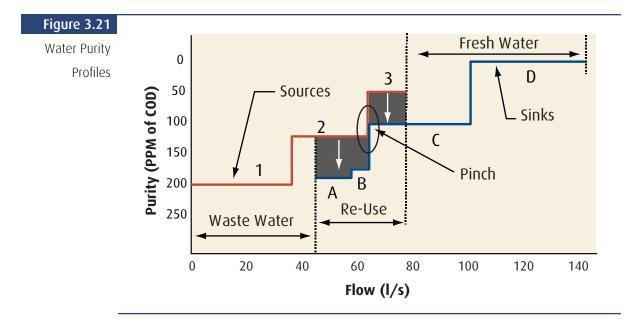
The overlap between the Sources curve and the Sinks curve indicates the scope for water reuse, and is limited by the pinch point where the two curves touch. Where there is no overlap, the profiles represent the freshwater consumption (on the right) and the wastewater generation (on the left).
