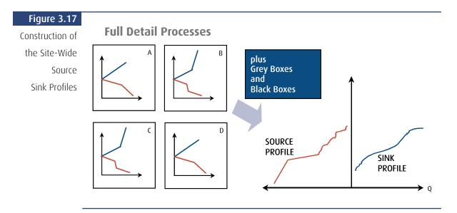
This is not the same as simply combining all the stream data for the various processes into a single data set. That would allow for every conceivable integration possibility across the site, usually a far from realistic scenario—constraints such as distances, controllability, flexibility, etc. reduce the number of possible matches to recover heat between two processes.
