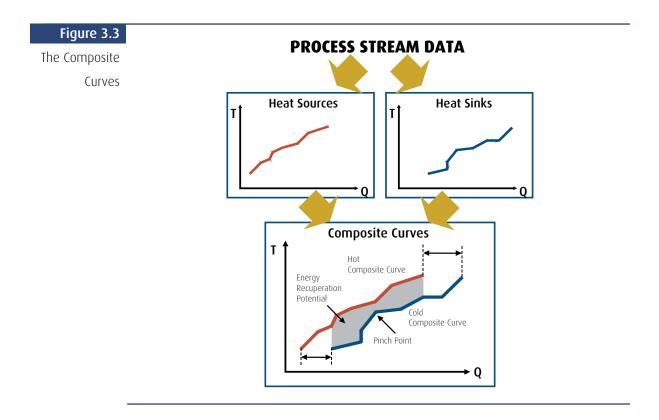
Constructing the curves requires only a complete and consistent heat and mass balance of the process in question. Data from the heat and mass balance are first used to define process streams in terms of their temperature and heating or cooling requirements As discussed in *Section 2.2*, this data may be produced from one or all of the following:
