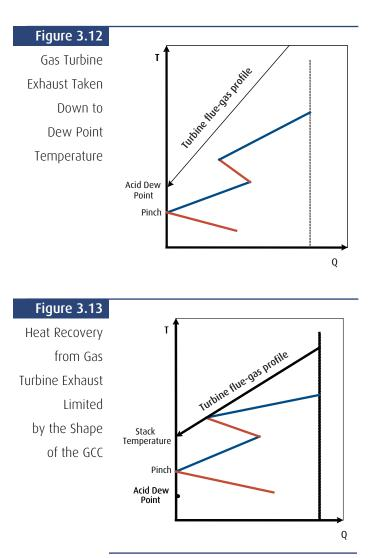
In summary, if a heat engine is placed across the process pinch, there is no benefit whatsoever from integration. Compare this with the potential of achieving 100% efficiency in the generation of useful work.
