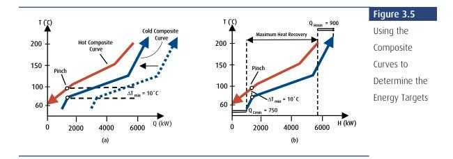
The overlap between the composite curves shows the maximum possible processheat recovery (as shown in *Figure 3.5(b)*), indicating that the remaining heating and cooling needs are the minimum hot utility requirement ( $Q_{Hmin}$ ) and the minimum cold utility requirement ( $Q_{Cmin}$ ) of the process for the chosen  $\Delta \Gamma_{min}$ . In this example, the minimum hot utility ( $Q_{Hmin}$ ) is 900 kW and the minimum cold utility ( $Q_{Cmin}$ ) is 750 kW.
