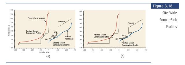
The optimization of steam levels only has significance in a grassroots design, or if the different levels are generated from the exhaust of steam turbines. In the above example, generating additional high-pressure steam would result in much more generation than consumption. To achieve savings, therefore, the high-pressure steam would have to be passed through a turbine to generate a lower-pressure steam at a level where there is a demand while generating power.
