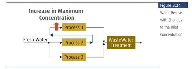
Projects to modify the water network are mostly defined at this stage. They mainly involve simple piping modifications, but will normally lead to significant water savings.
