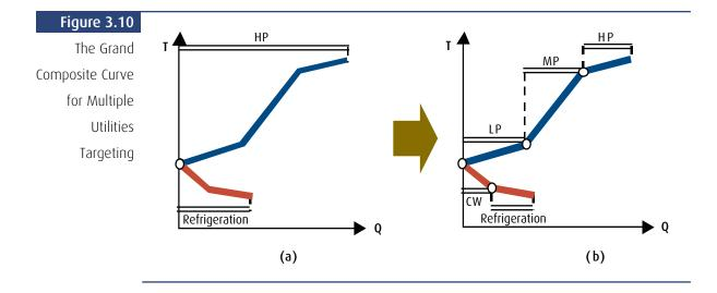
The target for LP steam (the less costly hot utility) is first set by plotting a horizontal line at the LP steam temperature (shifted) from the y-axis until it touches the grand composite curve. The MP steam target then follows in a similar way. The remaining heating duty is finally satisfied by HP steam. This reduces HP consumption in favour of MP and LP steam, thus minimizing total utility cost. A similar construction below the pinch maximizes the use of cooling water over refrigeration.
