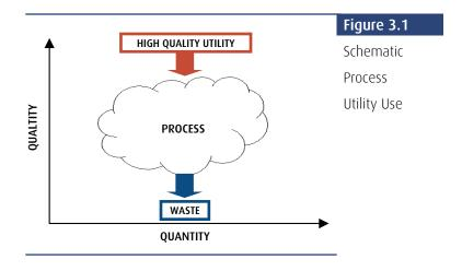
the quality required and the quality offered. In the context of utility management, the commodity may be heat, with its quality measured as temperature; or it may be water or hydrogen, the quality of which would be purity or pressure, for example. By maximizing the match between supplies and demands, we minimize the import of purchased utilities (*Figure 3.2*).
