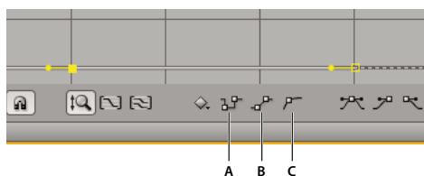
Interpolation buttons in the Graph Editor A. Hold B. Linear C. Auto-Bezier
