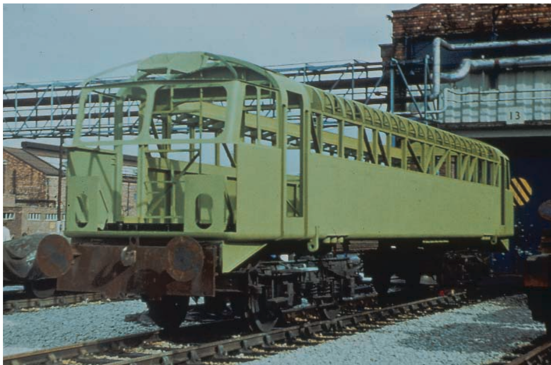
RIGHT: A rare view of a Class 87! In February 1973, the life of 87004 was just starting as the bodyshell stood at Crewe Works awaiting fitting out. COLIN J. MARSDEN
