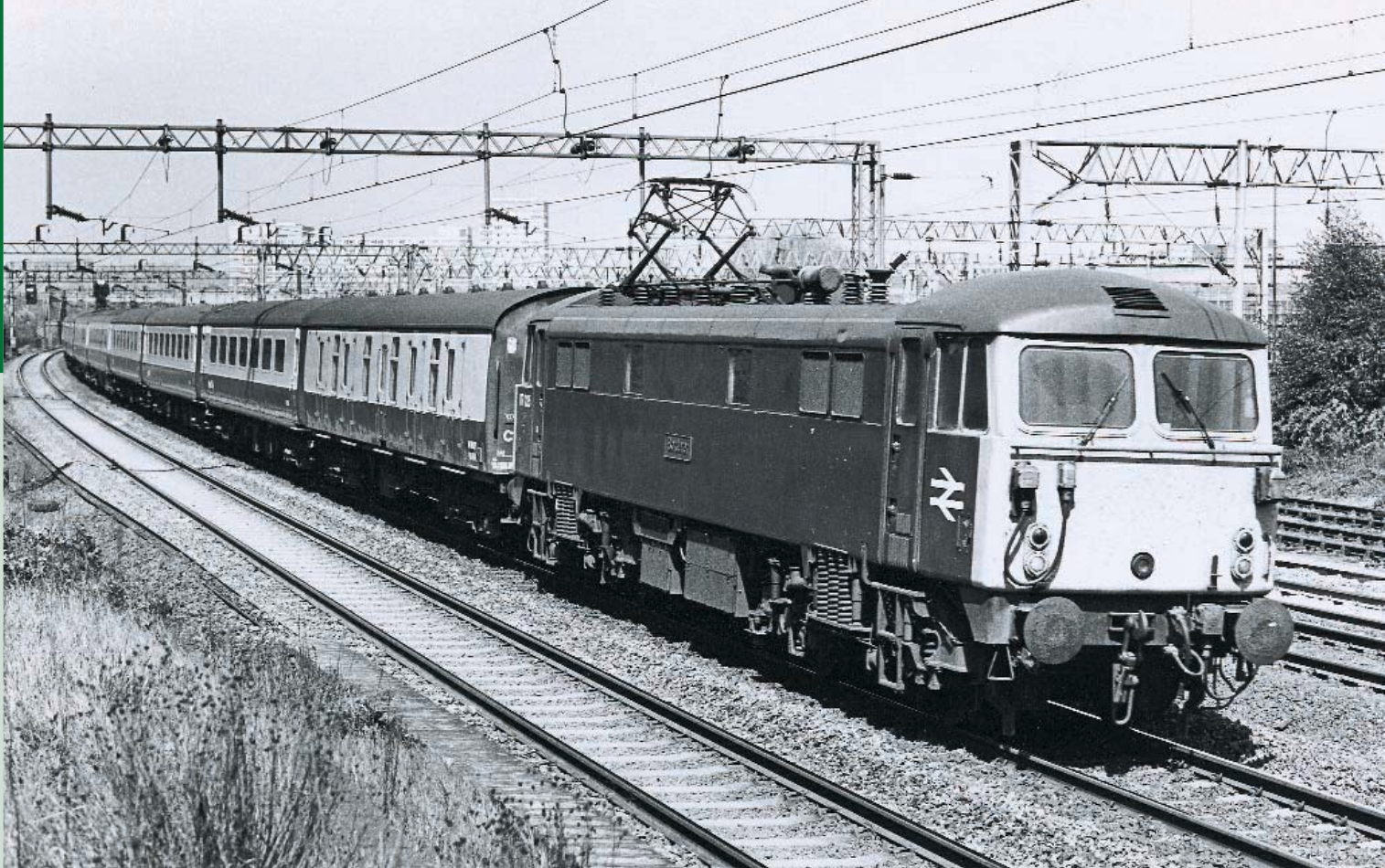
ABOVE: On 12th May 1980, Class 87 No. 87025 County of Cheshire heads along the final few miles of the West Coast Main Line at Willesden with the 06.00 Carlisle-Euston service. The photograph shows the original crossarm pantograph design which provided a maximum speed of 90mph and later 100mph. COLIN J. MARSDEN
