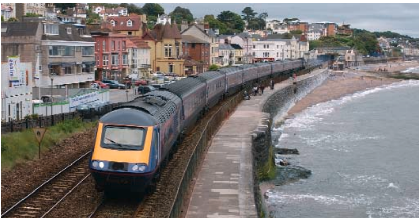
ABOVE: Recently released from Brush Traction at Loughborough, Class 43 No. 43009 has been re-engined as part of Angel Train's HST life extension programme. The power car, together with 43004, has been fitted with an MTU 16V4000 engine as part of a project jointly funded by Angel Trains and First. On one of its first loaded test runs, No. 43009 with 43022 on the rear passes Dawlish on 2nd June, bound for Plymouth. RICHARD TUPLIN
