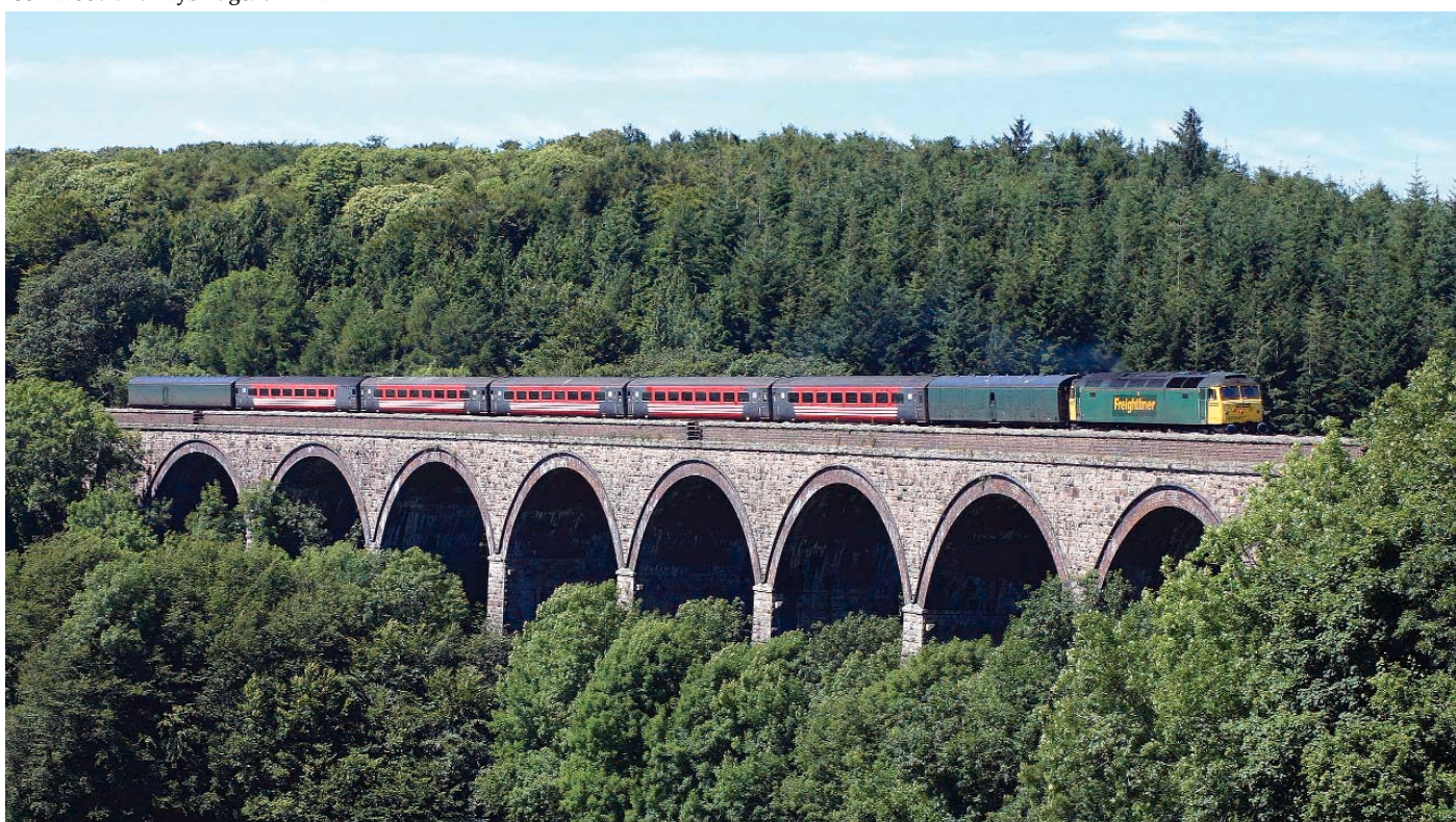
BELOW: On Thursday 14th July, First Great Western exchanged several ex-Virgin Mark 3 HST coaches between Minehead (on the West Somerset Railway) and Laira depot at Plymouth. Freightliner Heavy Haul provided the traction in the form of Class 47 No. 47150. The locomotive is pictured with the return trip, 5Z49 15.06 Laira - Bishops Lydeard, conveying coach Nos. 44068, 42305, 42304, 42303, 42302, crossing Blachford Viaduct between Cornwood and Ivybridge. SAM FELCE
