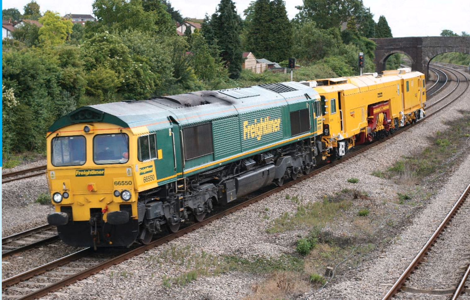
ABOVE: Class 66/5 No. 66550 is pictured at Magor heading west with the new Plasser & Theurer Dynamic Track Stabiliser machine, No. DR73112, heading to Margam for final commissioning. Of note are the yellow squares behind the cab windows on the loco. This is a new addition by Freightliner to allow drivers to easily distinguish DFRT locos from those in the DFHH fleet. CHRIS PERKINS
