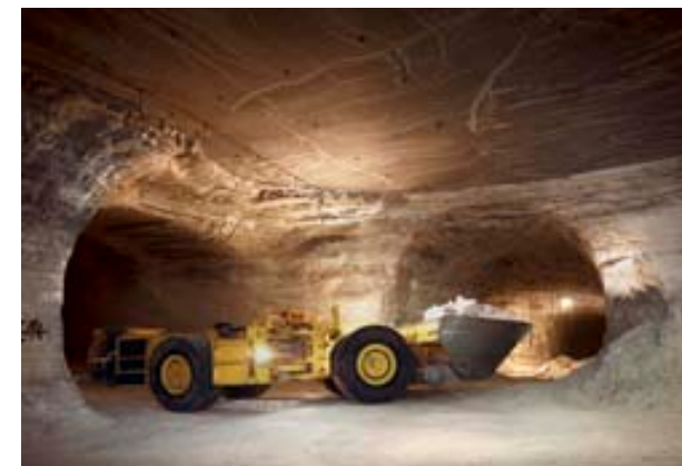
In their huge shovels, robust wheel-mounted loaders transport up to 20 tonnes of mined crude salt, the so-called debris, to the filling point in the mine. There, the chunks of salt are broken in a crusher before they are transported on long conveyor belts to the mine shaft and then to the surface.
