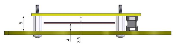
With this limitation the gap between baseboard topside components and module bottom side components is 0.5 mm.
