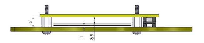
If the baseboard is using the connector with 8 mm stacking height the clearance between the baseboard and the bottom surface of the module's PCB is 8 mm. Components placed on the baseboard topside underneath the module shall be limited to a maximum height of 4 mm with the exception of the mating connectors.
