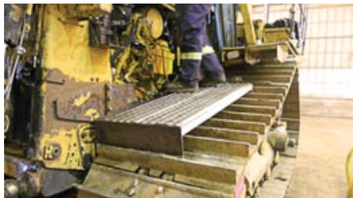
INVENTION TECH: Brent Einfeld shows the plywood prototype that led to the aluminum Trackwalker.
