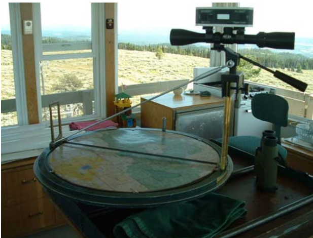
Figure 4. Improved Osborne firefinder with attached telescope and digital pitch readout. The photo shows the map disk inside the compass ring.
