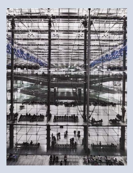
An equally efficient structural system is applied to the Airport's concourses. The engineers have developed these trusses in the form of an arch: one of the most efficient structural forms because it typically acts purely in compression. The gradual inward curvature of the five-point trusses shown below is used to combat the outward thrust exerted by the resultant arch.
