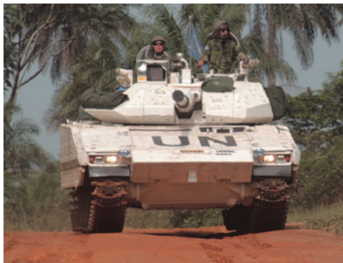
CV 9040 C with IED-Mine-Protection.
