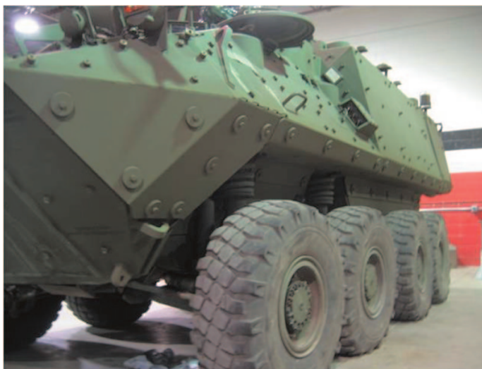
BISON with Heavy Blast-Fragments IED-Protection.
