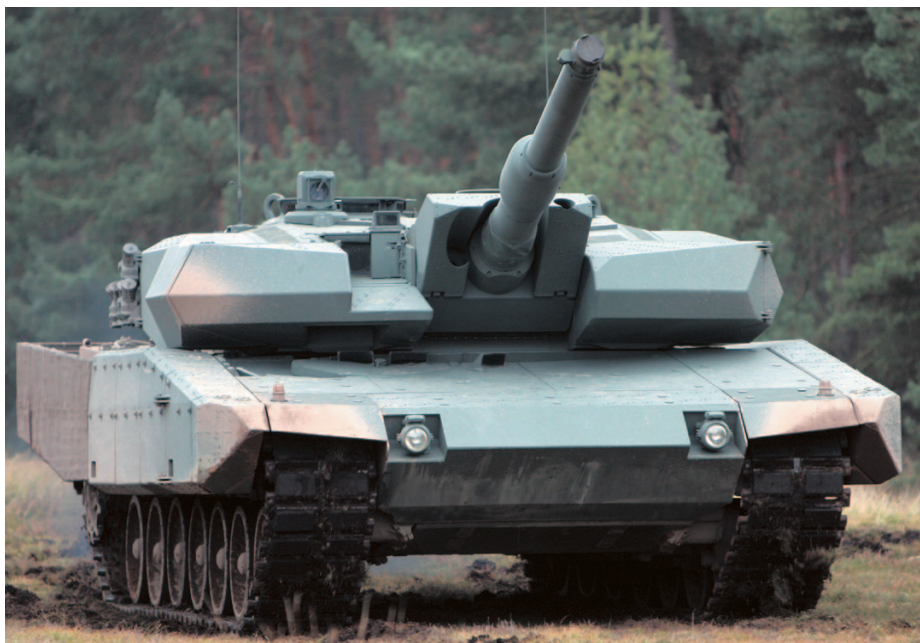
A LEOPARD 2 MBT fitted with IBD add-on armour including the AMAP-R ultra-light roof protection concept. (All photos: IBD Deisenroth)
