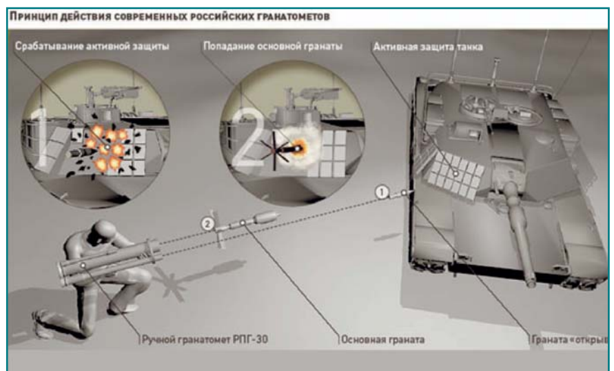
Figure 3: Operating method of RPG-30
