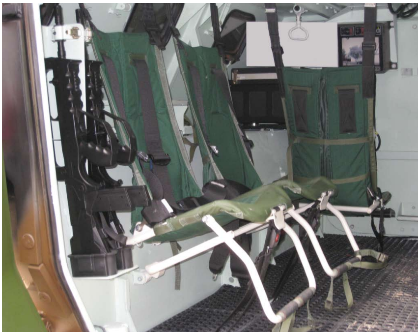
Mine protection seats and storage
