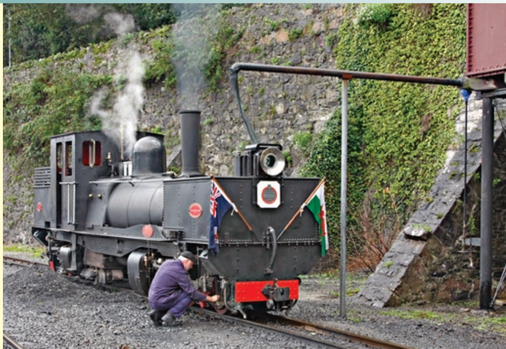
▲ The real thing. The world's first Garratt, built in 1909, pauses at Caernarfon between duties, on 6th September, for water and some judicious oiling. The plaque on the front celebrates the newly received IME 'Engineering Heritage Award'. All photographs by the author
