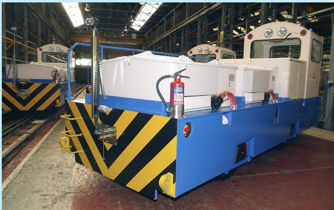
ABOVE: Three of the new battery locos for the Waterloo & City are pictured at Clayton Engineering Derby. METRONET
