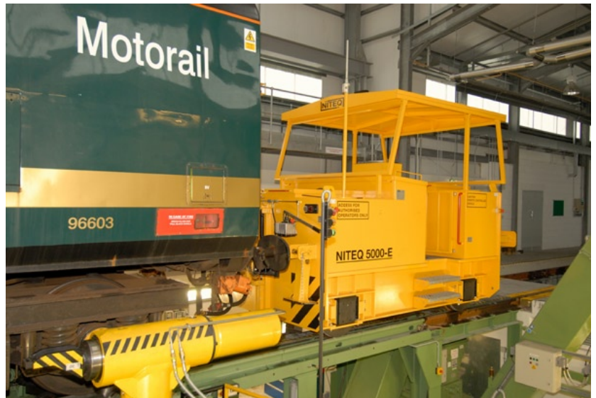
BELOW: The Niteq automatic self propelling locomotive used for powering vehicles into and away from the new Old Oak Common wheel lathe structure is seen on 19th February, with stored Motorail van No 96603 positioned ready for wheel profiling. BRIAN MORRISON
