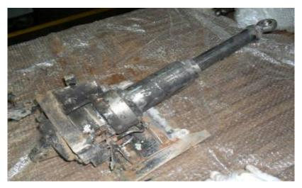
Photo 18: Leading Edge Actuator Assembly
