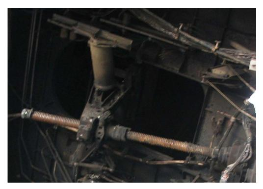
Photo 21: Photograph of Stabiliser Jack Screw
