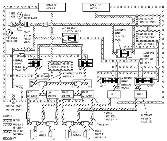
Diagram 8: Gear Retract Brake System
