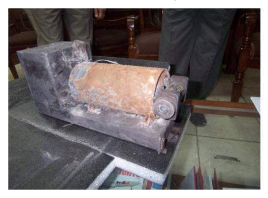
Photo 6: Damaged CVR Recovered From the Crash Site
