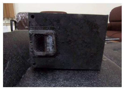
Photo 5: Connector of the CVR Damaged Due to Fire
