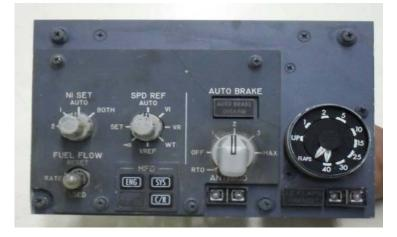
Photo 16: Brake Selector Panel and Flap Position Indicator
