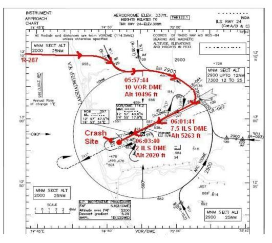
Diagram 2: Plan View of DME Arc Approach Leading to ILS
