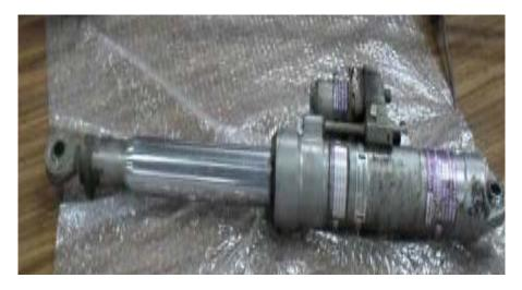
Photo 17: Leading Edge Flap Actuator
