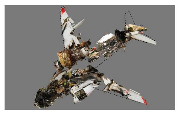
Photo 2: Photograph of the Re-arranged Wreckage
