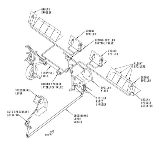
Diagram 7: Speedbrake Control System
