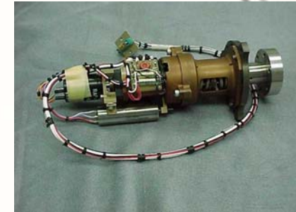
Composite Electromagnetic: Stepper Motor Coarse + Ceramic Fine
