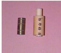
Piezoceramic Inchworm: Mechanism + Multilayer Stack
