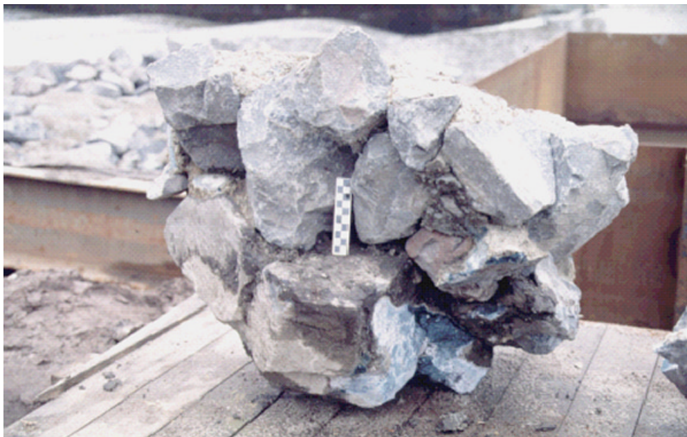
Figure 4.6. "Conglomerate" of partially grouted riprap, Federal Waterway Engineering and Research Institute, Karlsruhe, Germany. (43)
