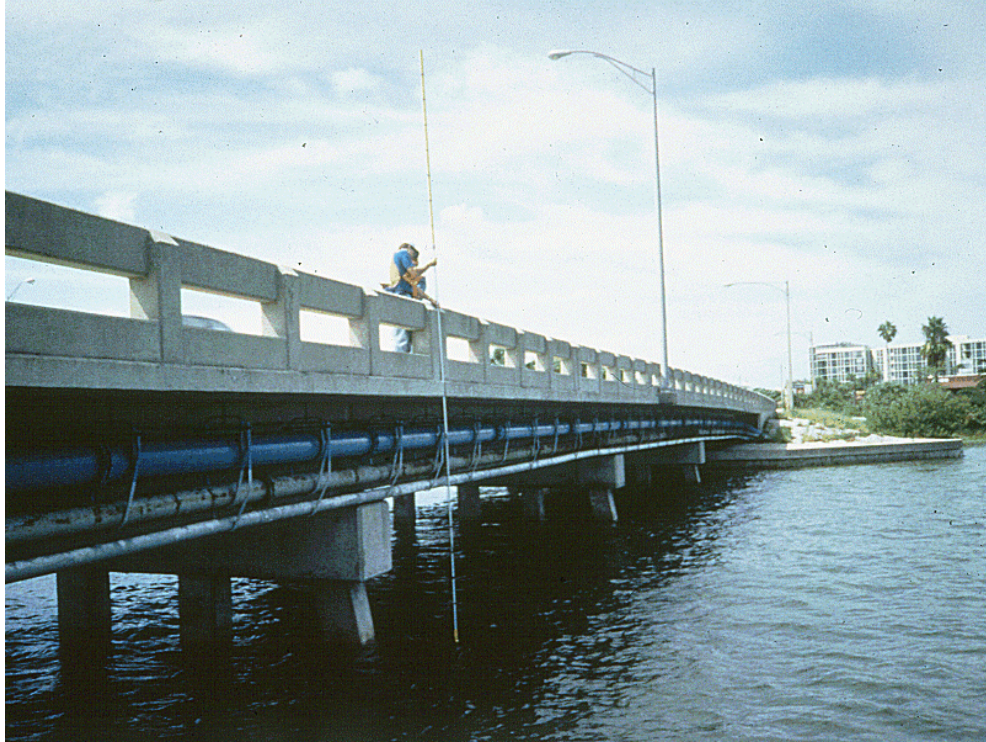
Figure 7.1 Sounding pole measurement.
