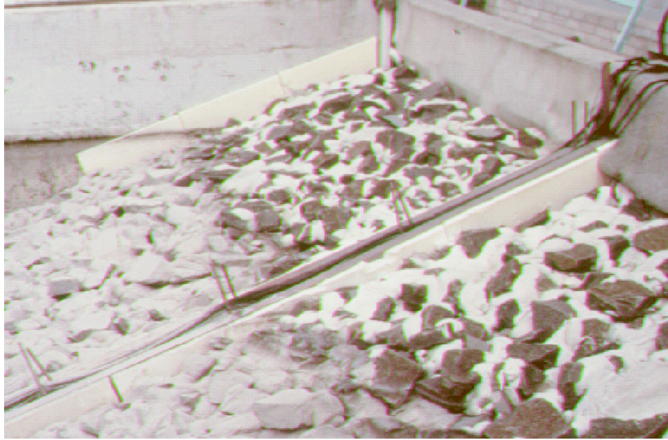
Figure 4.5. Partially grouted riprap undergoing testing at the Federal Waterway Engineering and Research Institute (BAW), Karlsruhe, Germany. (43)
