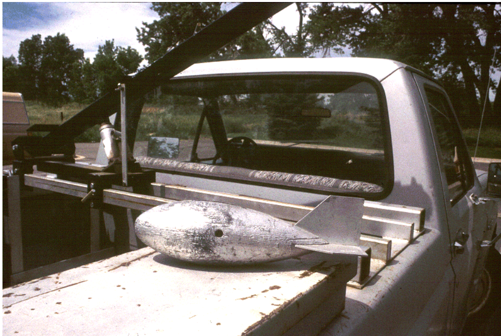
Figure 7.2. Lead-line sounding weight.
