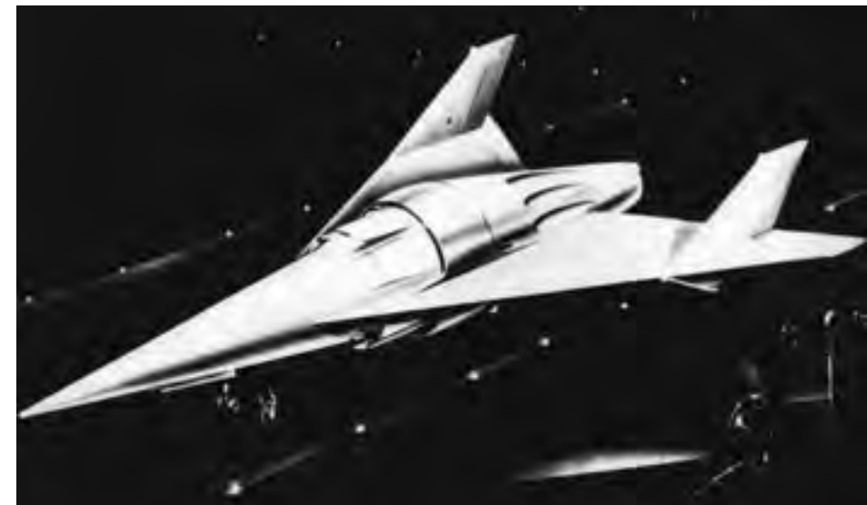
Republic's Aerospaceplane concept showed extensive engine-airframe integration. (Republic Aviation)
