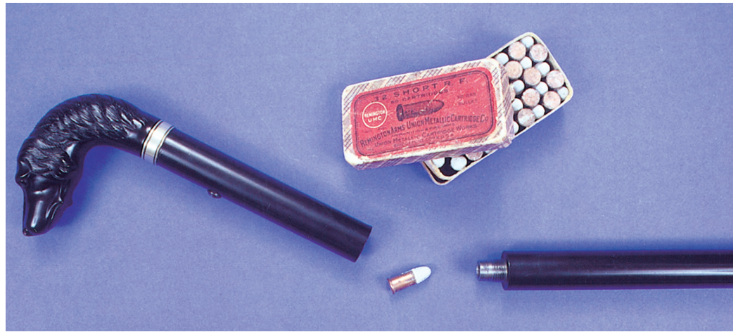
Figure 15. Loading the .32 rf cartridge rifle cane.
