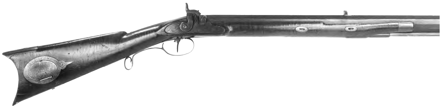
Figure 10. Three quarter view of the right side. Note the slivers missing from the fore end, and the expansion of the wrist from front to back.
