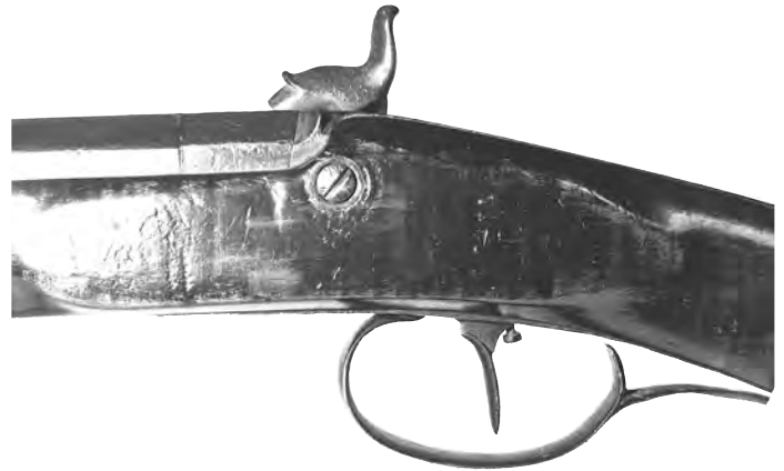
Figure 11. Close up of the left side breech area. Note the “slant breech” surface (just under the nose of the hammer) and the vestige of a flash fence on the tang block just behind it.
