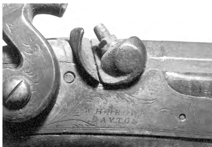
Figure 4. The name on the lock is W. H. BROWN/DAYTON which dates this component from 1827 to 1843. The design of the "snail" around the percussion nipple, which shows some sophistication, shortens this span to about 1835 to 1843, the time frame in which the gun must have been made.
