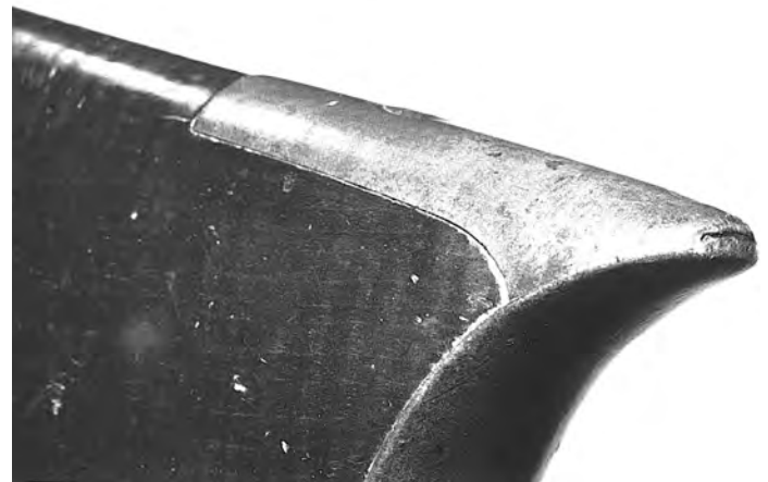
Figure 6. Break and seam in the butt plate heel indicating handcrafted construction.
