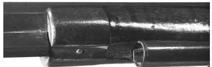
Figure 7. Fore end cap showing a fine seam where the front plate is joined to the collar, again indicating handcrafted construction.
