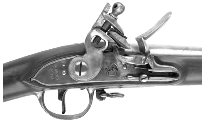
Figure 2. Typical lock markings on Henry manufactured musket.
