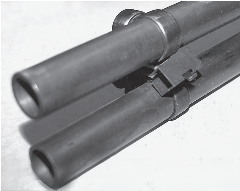
Figure 19. Maynard double gun patent applied to his gun from the muzzle end.
