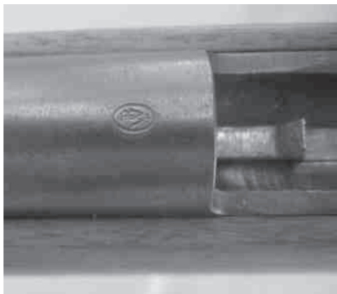
Figure 18. Winchester proof mark centered on the top of a Model 67 receiver.
