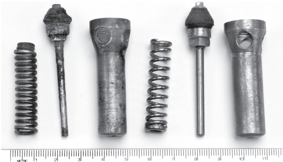
Figure 11. Girardoni Air Rifle, valve and brass valve springs, original (left) and reproduction (right).
