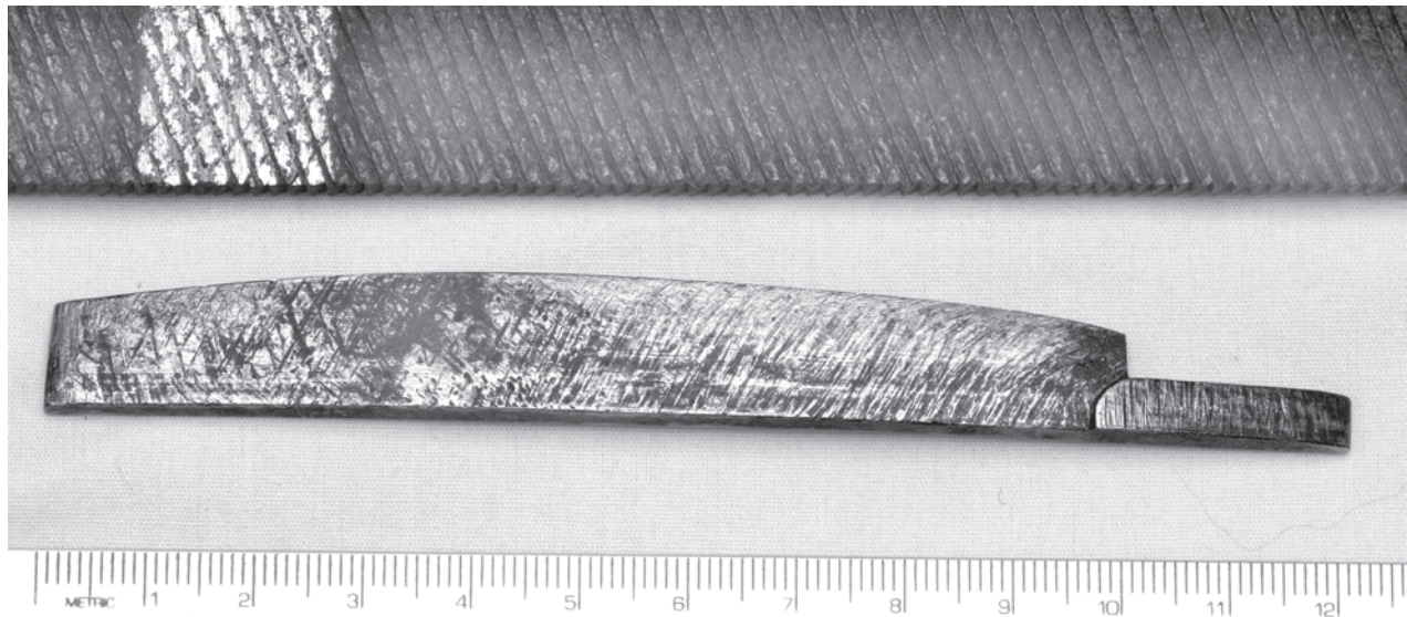
Figure 14. Girardoni Air Rifle, replaced main spring (bottom) and period ferrier's file (top) Matches description of repair effected by John Sheilds.
