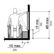
Unobstructed side reach with an allowable obstruction less than 10 inches (254 mm) deep.
