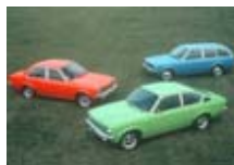
The three body variants of the Opel Kadett C: sedan, station wagon and coupe, 1973–1979.
