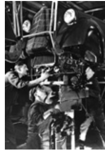
The wedding: final assembly by means of Opel's patented manufacturing process.
