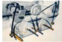
The Opel Safety System in the Astra F, 1992: seatbelt tensioner.
