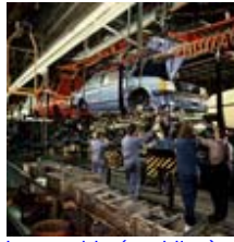
Final assembly (wedding) of an Opel Kadett D in the Bochum plant, 1979.
