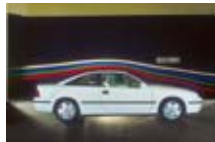
Wind-tunnel testing of the Opel Calibra, 1989.
