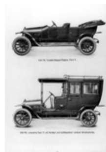
The two variants of the 10/24 hp Opel from 1911: a torpedo double phaeton and a covered limousine with a fold-down windshield.
