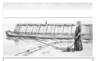
Figure 9 - Strapping a boat round a junction
