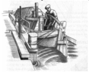
Figure 11 - Strapping a gate closed
