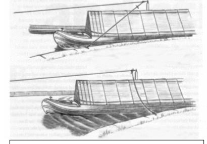
Figure 12 - Use of blocking pins
