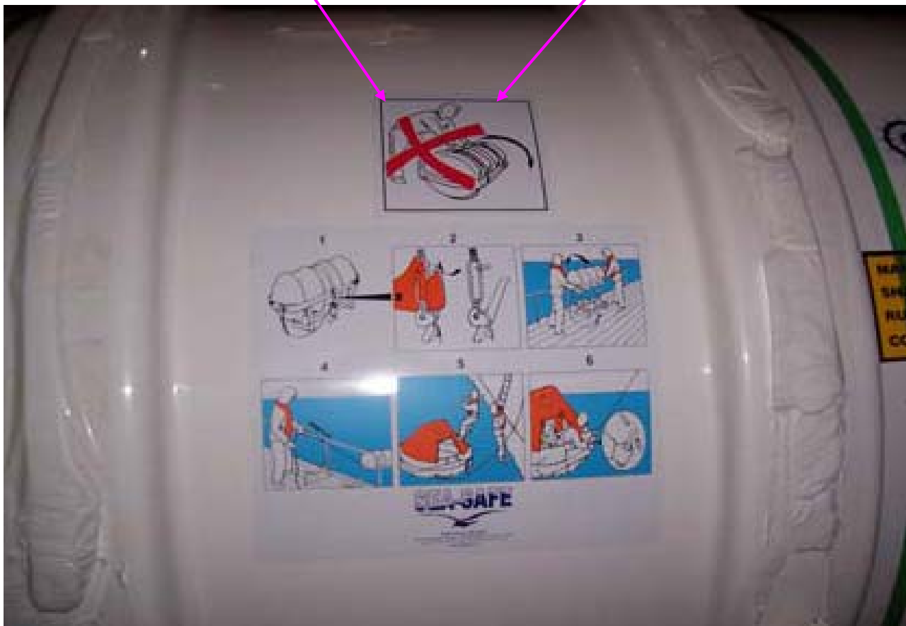
Site Photo 30. Close-up on instructions located on the life raft storage barrel (NOTE: ABOT personnel will have to decipher the instructions while trying to escape a potentially burning platform)
