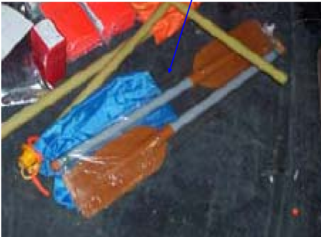
Site Photo 32. Enlarged view of the life raft oars, which appear to be made of plastic
