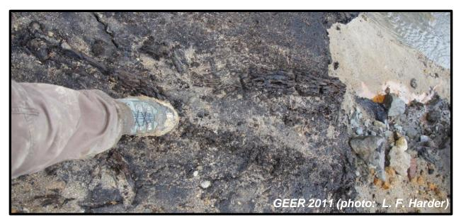
Figure 17: View of Old, Rotted Small Tree Trunks Embedded within Black Organic Foundation Residual Soil Exposed in Eroded Channel Downstream of Breach in Fujinuma Main Dam (N37.3022°, E140.1959°, April 23, 2011)
