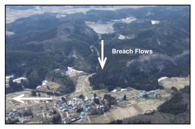
Figure 35: Aerial View of Breach Flow Path below Fujinuma Main Dam towards Naganuma (adapted from Japanese National Institute for Land and Infrastructure Management, 2011)
