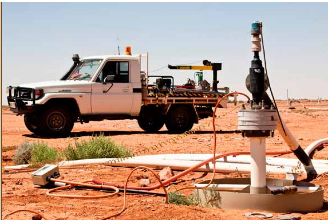
Production well at Beverley in situ recovery uranium mine, South Australia (Heathgate Resources)
