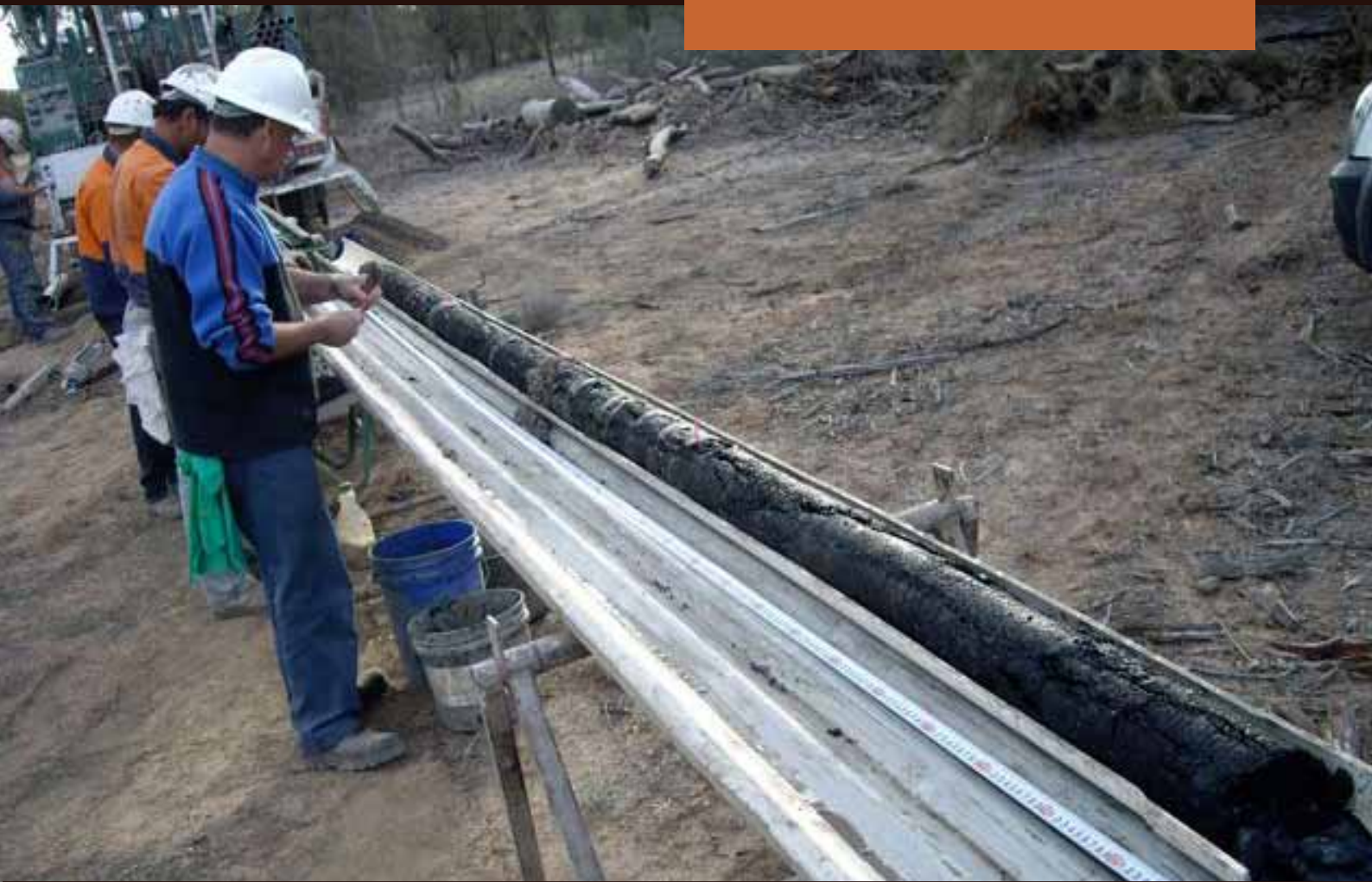
Logging core at Cameby Downs coal mine Queensland (Syntech Resources Pty Ltd)
