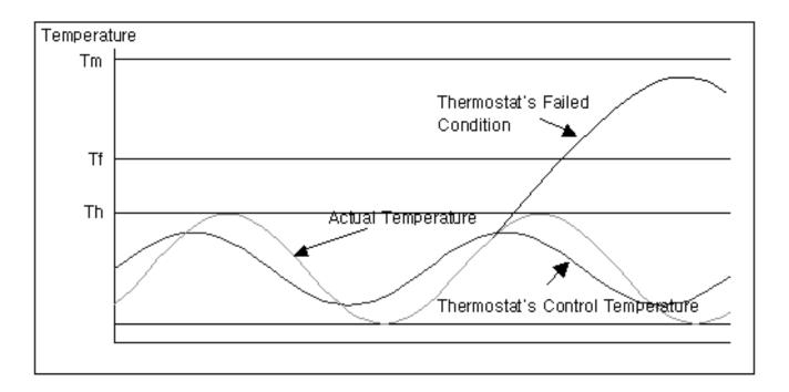
Each TCO has specific electrical and temperature ratings. Each TCO must be used within the prescribed ratings. These ratings include Rated Function temperature(TF) ,Holding Temperature(TH), Maximum Temperature (TM), and the electrical ratings.
