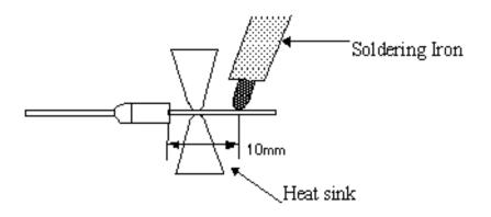
\* Mechanical security must not depend on solder alone.
