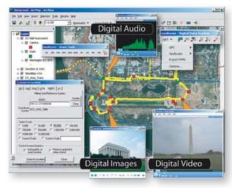
The Digital Data Tracker extension downloads GPS receiver track logs and waypoints as layers in ArcGIS Desktop. Using the downloaded GPS information, data collected in the field (digital images, video clips, digital audio, etc.) can be automatically georeferenced and plotted in the ArcGIS Desktop display. Click on the points to access the data. Hours of field data collection can be processed in seconds.
