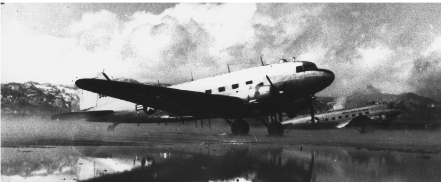
This C-47 is not quite what it appears to be. It was used by the 6147th TCG as an airborne radio relay aircraft.
