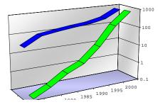
Figure 1. The total area of astronomical telescopes in  $m^2$ , and CCDs measured in Gigapixels, over the last 25 years. The number of pixels and the data double every year.
