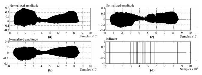
**Fig. 3.** Result of *gruppett* synthesis employing three different methods: a) synthesized *gruppett* using Glottal Pulse Model, b) synthesized *gruppett* employing single fragment of original glottal pulse, c) synthesized *gruppett* employing multiple fragments of original; glottal pulses using correlation technique, d) indicator function, showing places where glottal pulse shape was changed during synthesis presented in part (c)
