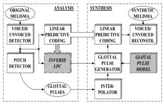
**Fig. 2.** Two cases of melisma synthesis/restoration in the one scheme. First case employs Glottal Pulse Model indicated by right grey dotted box. Second case uses Inverse LPC block shown as a grey dashed box at left
