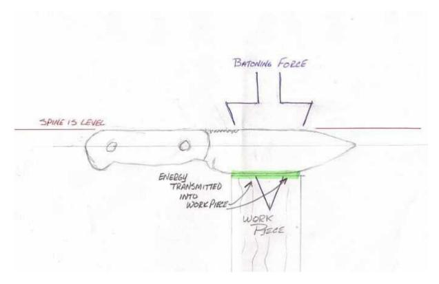
The force of the blows on the spine of the knife drives it directly down into the work piece. It's almost impossible to break a knife like this. The problem comes up when the blade has been driven flush with the work piece making it impossible to hit the spine.
