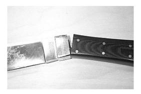
I believe that knives break because the act of batoning puts abnormal strain on the tang of the knife. If you use the correct technique almost any knife can be used to baton, including folding knives although I strongly recommend against doing so.
