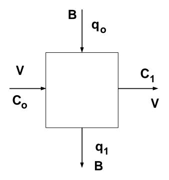
At a given time *t* when the carbon is separated the following mass balance can be written:
