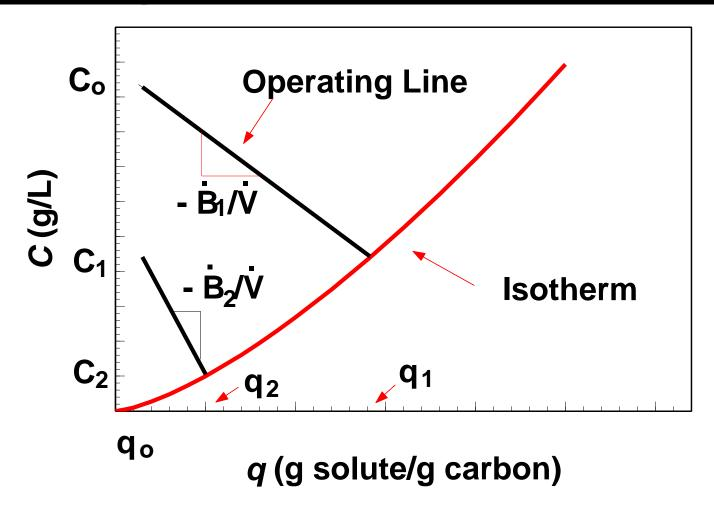
In this case fresh carbon is added to each stage of the adsorption process.
