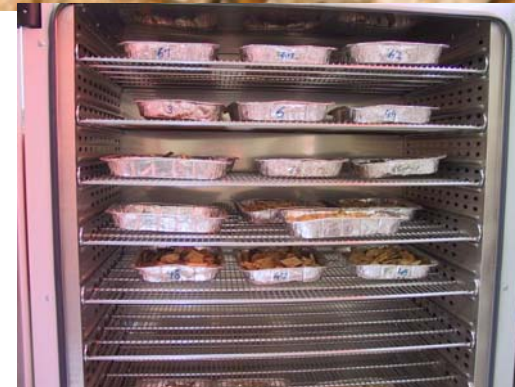
Drying oven, moisture content prEN 14774-1 – 3
