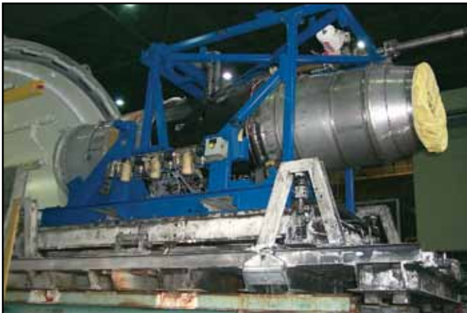
The AE3007H Engine for the RQ-4 Global Hawk being Installed in T-4.
