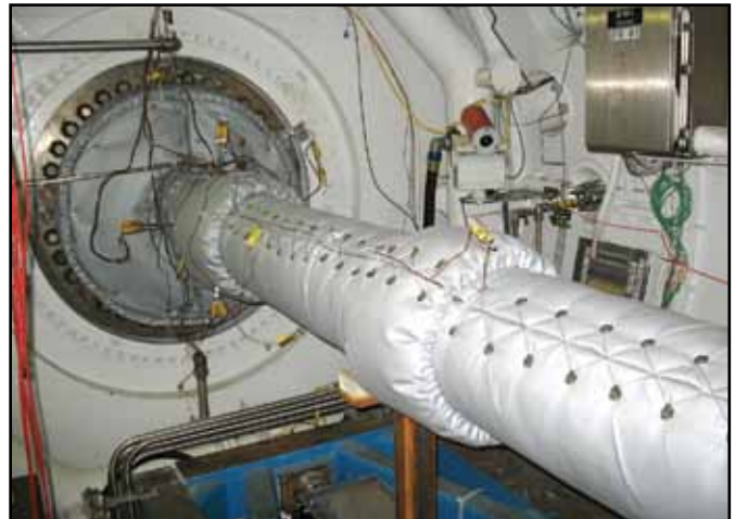
Insulation Blankets to Reduce Test Cell Heat Load in T-3
