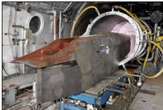
DARPA FaCET Test Article Installation
