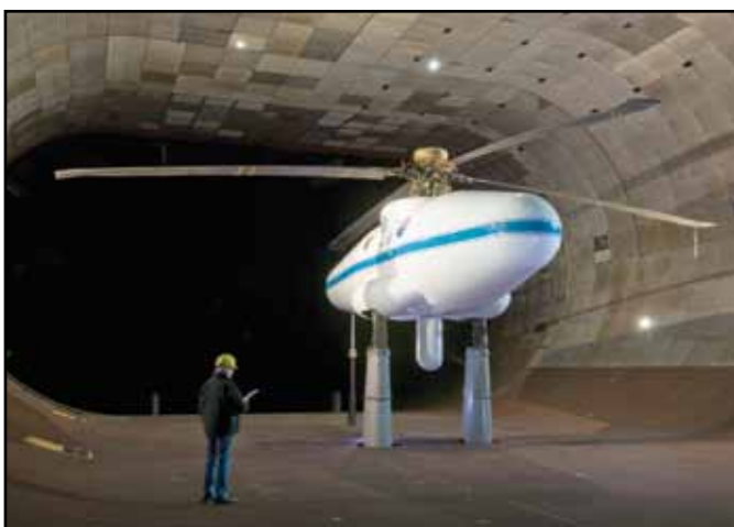
NASA/Army UH-60 Individual Blade Control Test on the Large Rotor Test Apparatus (LRTA)
