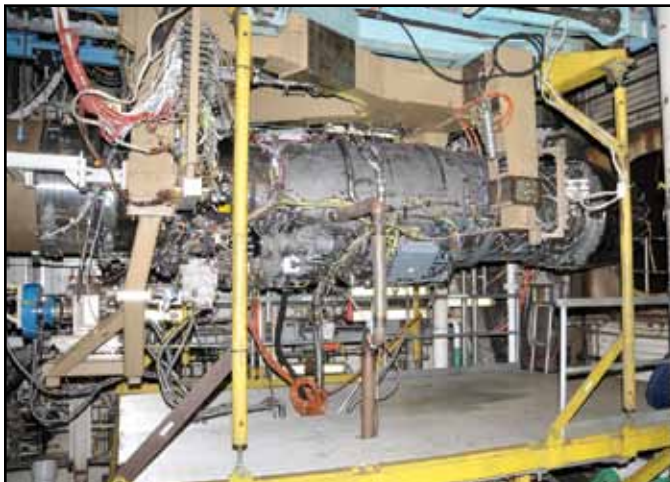
The F135 Engine for the F-35 Lightning II Aircraft Installed in C-1
