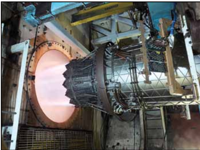
The F135 Engine for the F-35 being Tested in Test Cell J-2
