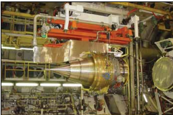
The XF7-10 Engine for the Japanese P-1 being Installed in C-2
