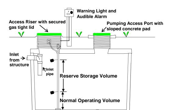
Figure 1. Longitudinal-Section of Typical Holding Tank Sewage System.
