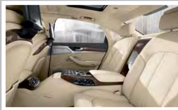
Rear seat package – two individual rear seats with reclining seat and foot rest
