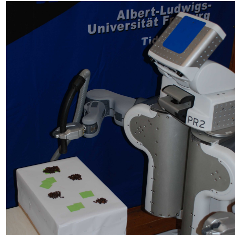
Fig. 1: Experimental setup. The PR2 cleans a table with a vacuum cleaner. Instead of cleaning the whole table, the robot observes the outcome of its actions, learns which features correspond to dirt, and cleans these regions.
