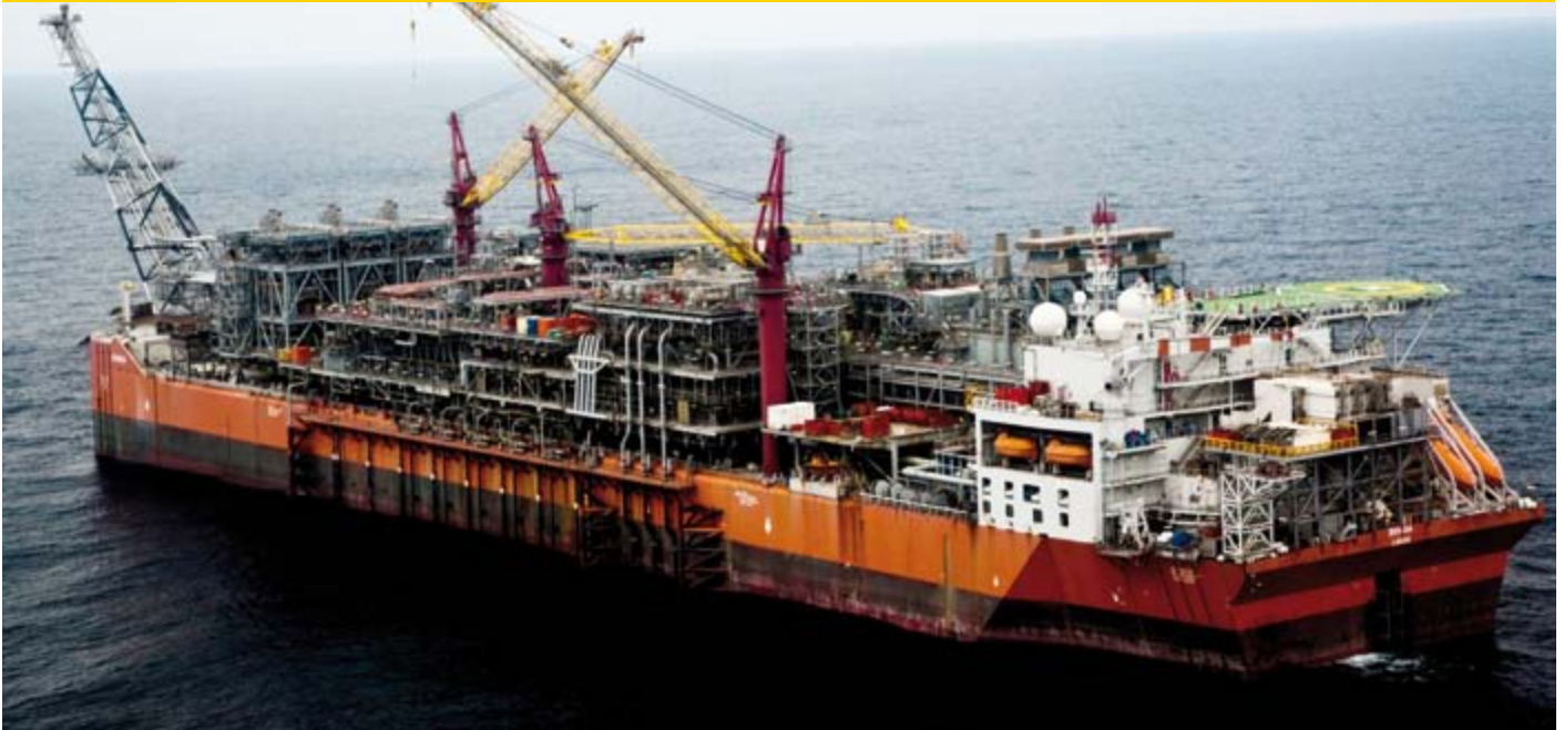
A side view of the Bonga Floating Production Storage and Offloading vessel (FPSO)
