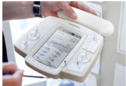
Figure 16.11. Using a foam model to refine control placement.
